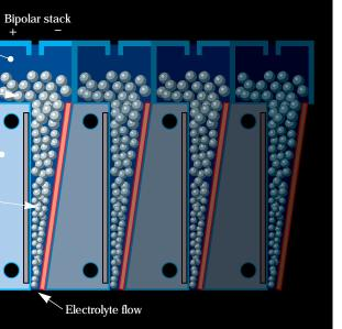
Figure 3. Zinc pellets are gravity fed from hoppers to cells.
