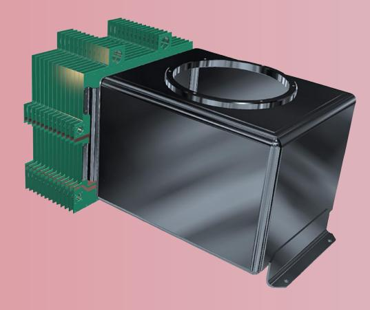
A recent road test at LLNL underscored the *zinc/air batterv's capacity to give electric* vehicles some of the attractive features of gas-driven cars: a 400-km range between refueling, 10-minute refueling, and highwaysafe acceleration.
