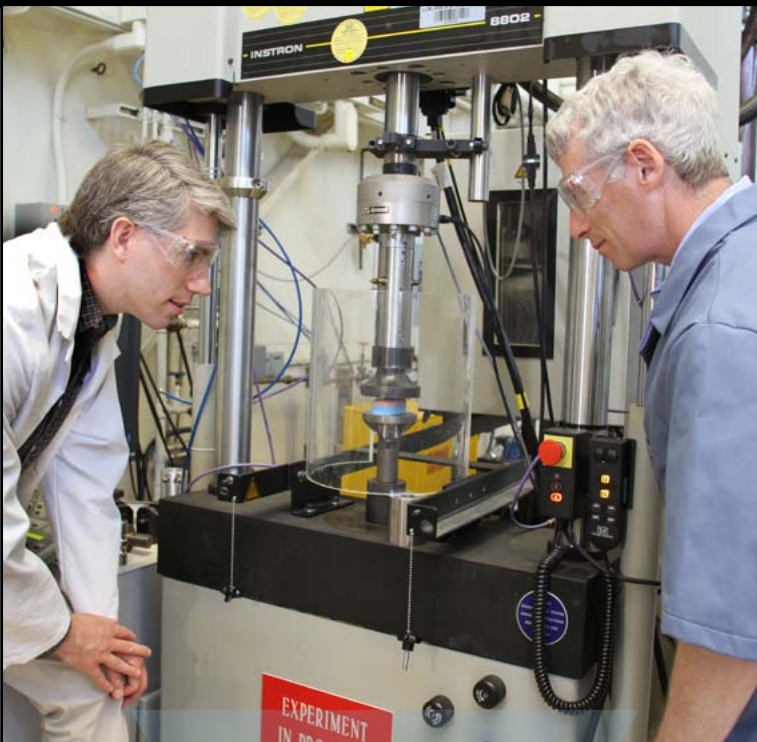
LLNL mechanical engineer Mike King (left) and physicist Willy Moss watch a compression test of a helmet pad.
