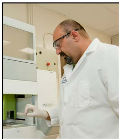
Pejman Naraghi-Arani holds one of the assay chips that the Nanostring Counter uses for detection and quantitation of RNA molecules.
