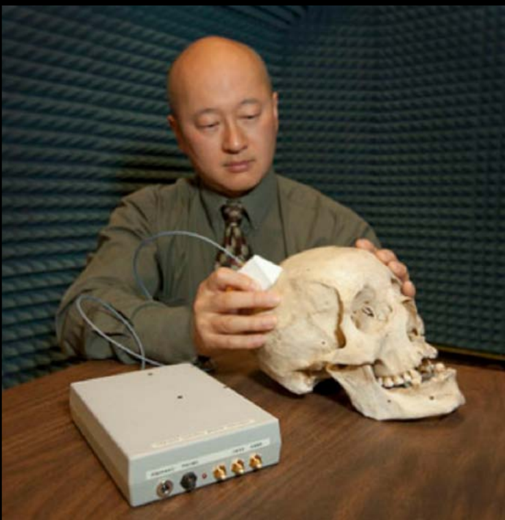
LLNL researcher John Chang tests a prototype intracranial hematoma detector on a human skull. Work on this project won an award for excellence in technology transfer from the Federal Laboratory Consortium.
