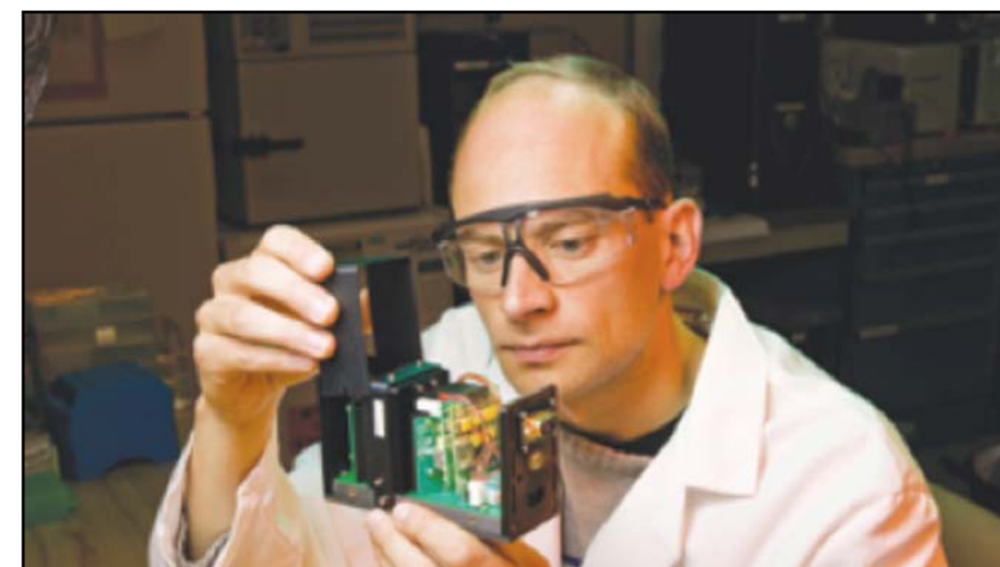
LLNL electronics engineer Vincent Riot holds the polymerase chain reaction module of the Environmental Sample Processor, a robotic biochemistry lab that can be placed in the ocean to analyze genetic material.
