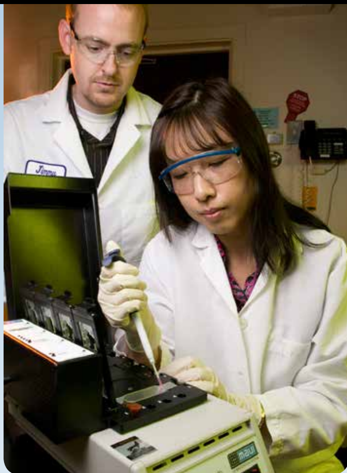
LLNL biologist Crystal Jaing loads a fluorescently labeled viral DNA sample onto the Lawrence Livermore Microbial Detection Array as fellow biologist James Thissen watches.
