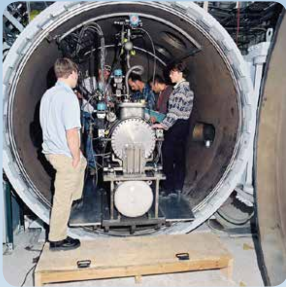
JASPER staff inside the outer containment vessel inspect the sealed inner chamber, which houses the plutonium target.
